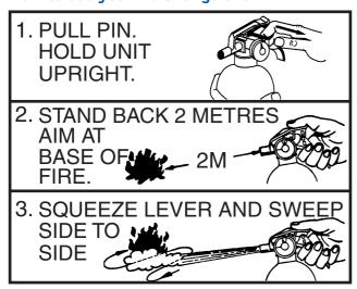
Study nameplate instructions and unit carefully to familiarize yourself with the operating instructions. Quell portable extinguishers operate by squeezing the lever. Each time the lever opens the valve, the stored pressure will force out some of the extinguishing agent. If the lever is not released the entire contents will be discharged.
