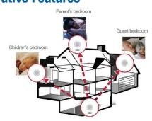
Interconnected alarm detects fire somewhere in the home and triggers other Quell interconnected alarms in the network.
