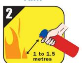
Hold can 1 to 1.5 metres from fire and aim at the base of fire
