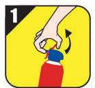
Place finger on trigger when removing tab from the trigger assembly
