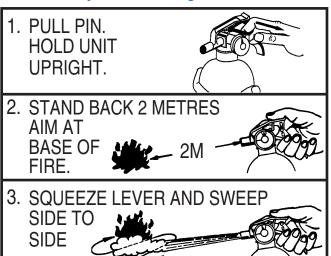
Study nameplate instructions and unit carefully to familiarize yourself with the operating instructions. Quell portable extinguishers operate by squeezing the lever. Each time the lever opens the valve, the stored pressure will force out some of the extinguishing agent. If the lever is not released the entire contents will be discharged.
